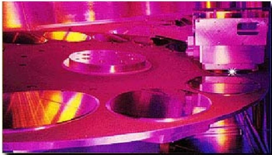
Ion Implanter Water Handling Mechanism
