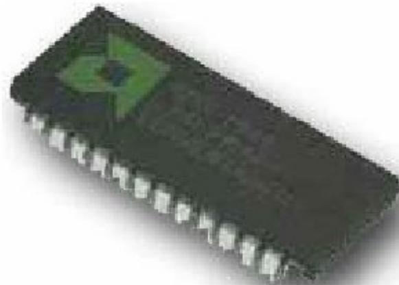
DIP (Dual In-line Package) Device
